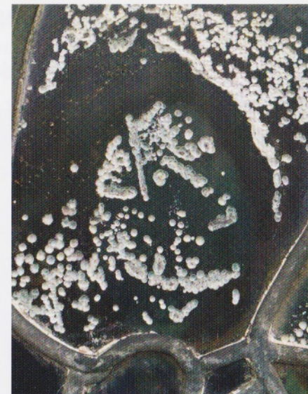
Internal and external views of pitting corrosion on the face of an angel.
